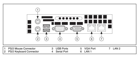
Figure 3-1 shows the rear panel layout of the NI 8352/8353.
